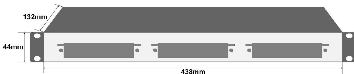
Figure 2.2.1 View of a remote 1U rack
